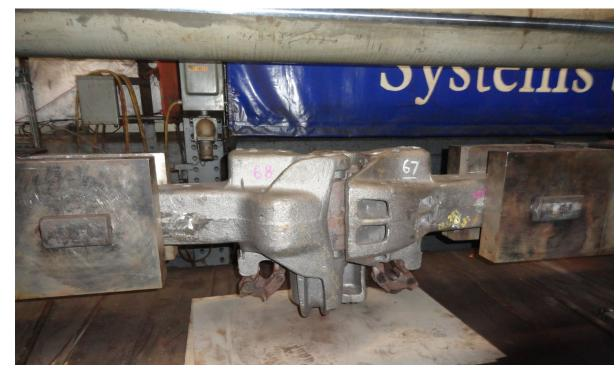
Dynamic fatigue machine built by Amsted Rail will be used to evaluate the design
