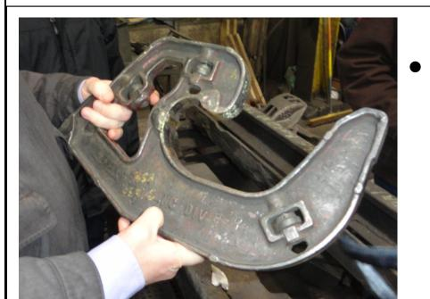
Knuckles will have to fit standard AAR gauges, such as the A-10 contour gauge (shown left)
